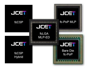
Our fcCSP packages form a subgroup of the Flip Chip package family of the form factor known as Chip Scale Packages (CSP). We offer a complete fcCSP portfolio of high to low-end leading edge packages for all mobile applications including standard fine pitch fcCSP packages, hybrid flip chip and fcPoP including Bare Die fcPoP, Interposer POP and Molded Laser PoP (fcPoP MLP).
